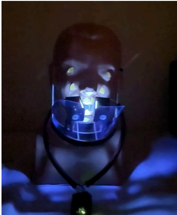
Photographic images of pieces of colorimetric dosimetry card affixed to the face and eyes of a human manikin with the Eden Park mask.
