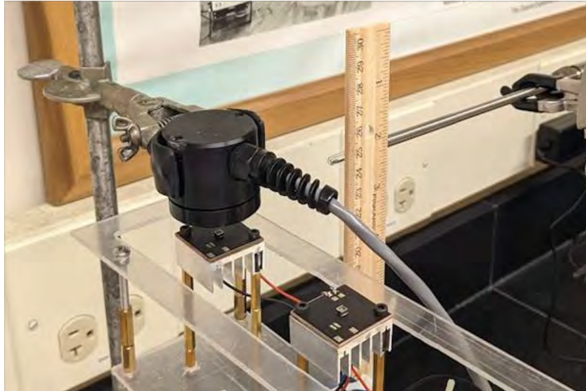
Calibration of 280 nm UVC LED
